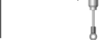
5) Move the shock shaft in and out a few times and then push it all the way in. It should be easy to push the shaft in until the eyelet hits the body.
