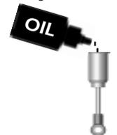
4) Thread the Eyelet Cap assembly onto the Shock Body until it is hand tight. Oil should seep out of the bleed hole in the Threaded Cap.
