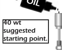
2) Slowly move the shaft up and down several times to allow air bubbles to escape to the top.
