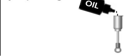
8) If the shock rebounds too fast, or you cannot push the shaft in until the eyelet hits the body, there is too much oil. Loosen the cap about 2 full turns and pump out a small amount of oil by pushing the shaft in. Retighten the cap and try steps 5-6 again.
